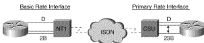
Figure 11-5: Connectivity to ISDN using BRI and PRI.
