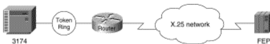
Figure 5-22: QLLC conversion supports SNA end-station connections over Token Ring and X.25 networks.
