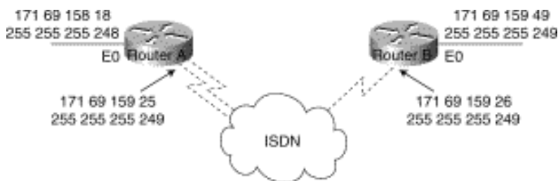
Figure 10-7: Example of dial backup over ISDN.
