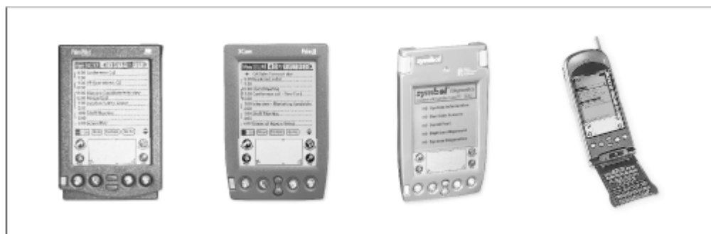
Figure 1- 2. Differences in physical design of Palm OS handhelds (from left to right): PalmPilot, Palm III, Symbol SPT 1500, and Qualcomm pdQ
