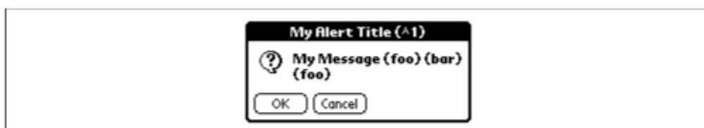
Figure 5-7. An alert displayed with FrmCustomAlert ; note that FrmCustomAlert doesn't replace strings in the title
