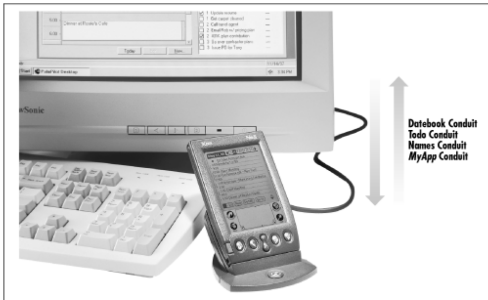
Figure 2- 1. Conduits control the exchange of information
